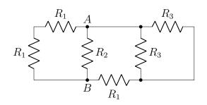
$$R_1 = 1\,\Omega \qquad \qquad R_2 = 2\,\Omega \qquad \qquad R_3 = 6\,\Omega$$
