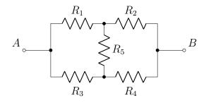
$R_1 = 1 \Omega \qquad R_2 = 2 \Omega \qquad R_3 = 3 \Omega \qquad R_4 = 4 \Omega \qquad R_5 = 5 \Omega$
