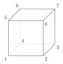
How large is the equivalent resistance between the corner points 1 and 7. Note: Use symmetry and potential equality!
