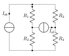
$R_1 = 10 \,\Omega$   $R_2 = 20 \,\Omega$   $R_3 = 30 \,\Omega$   $R_4 = 40 \,\Omega$   $I_{s5} = 5 \,A$   $I_{s6} = 6 \,A$
